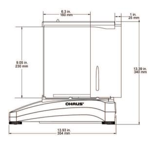
Figure 9-1. Draft Shield models
